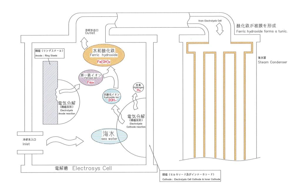
B: A ferric hydroxide tunic is formed in the inside of piping for corrosive protection. 防食
