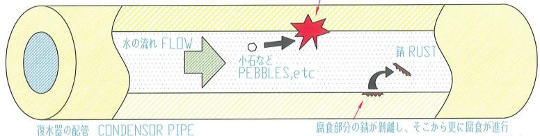
The rust of the corrosion partial surface exfoliates and it corrodes further from there.
